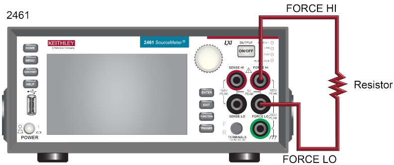
Figure 19: Model 2461 2-wire front-panel connections
