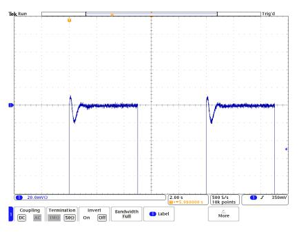
Figure 11: Digital filter aberrations (about 2.5% of V<sub>p-p</sub>)
