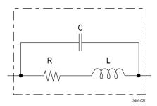
Figure 18: SMT resistor model
