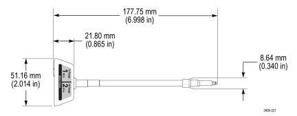
Figure 24: Probe tip adapter dimensions
