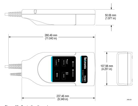
Figure 22: Controller dimensions
