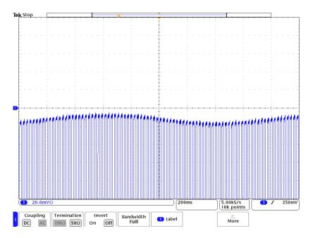
Figure 10: Digital filter aliasing
