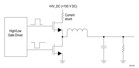
Figure 17: High side current shunt
