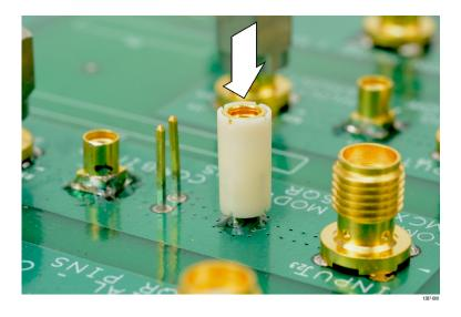
Figure 31: Pushing the MMCX-to-0.062-inch (1.57 mm) adapter in place
