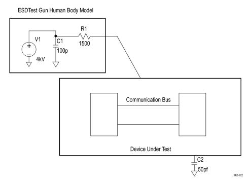
Figure 19: ESD discharge test example
