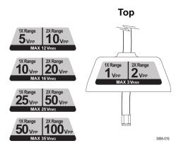
Figure 13: Top sensor tip labels
