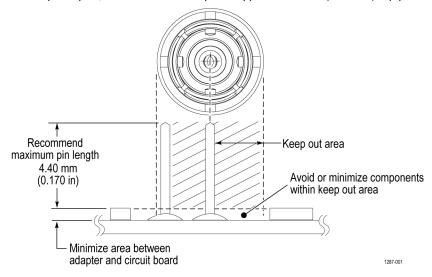
Figure 33: Adapter clearance requirements
