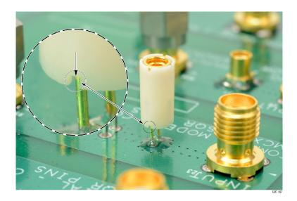
Figure 30: Lining up the MMCX-to-0.062-inch (1.57 mm) adapter on the circuit board After lining up the adapters gently push down on the adapter to seat it in place on the circuit board.
