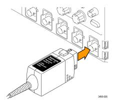
Figure 6: Connect the Comp box to the oscilloscope
