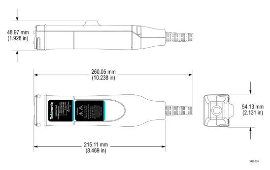
Figure 21: Sensor head dimensions without probe tip cover
