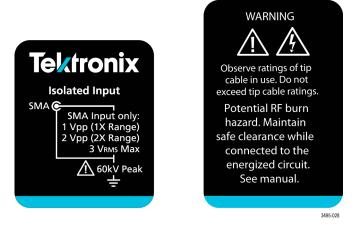
Figure 4: Labels on the sensor head
