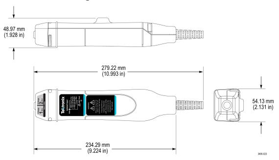
Figure 20: Sensor head dimensions with probe tip cover
