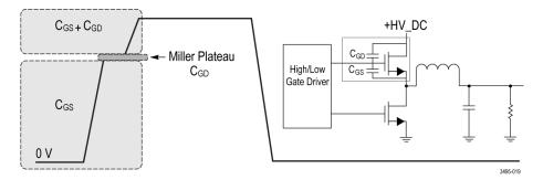
Figure 16: High-side turn-on characteristics
