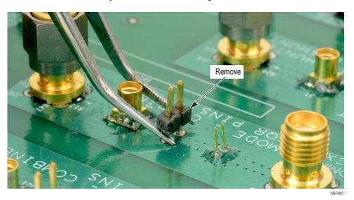
Figure 34: Removing the header from square pins on the circuit board
