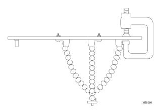
Figure 26: Installing the flexible tripod under the DUT.
