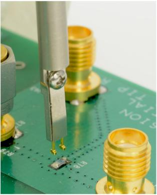
Figure 35: Using the soldering aide to install the square pins on the circuit board
