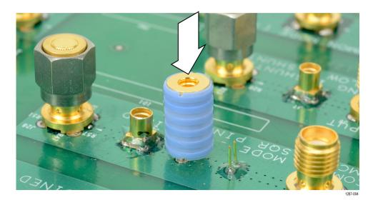
Figure 32: Pushing the MMCX-to-0.1-inch (2.54 mm) adapter in place
