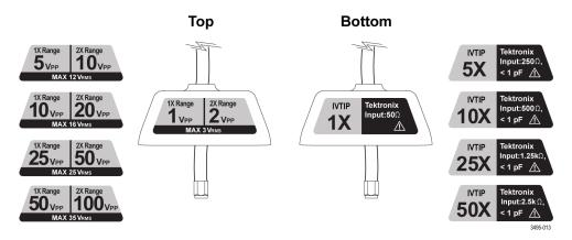
Figure 5: Sensor tip cable top and bottom labels
