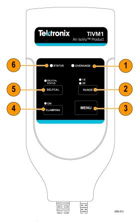
Figure 3: Controller indicators and buttons
