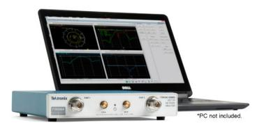
An independent RF source and three RF receivers for each port of the TTR500 enable you to take high-accuracy magnitude and phase measurements with a 1-port or 2-port device under test (DUT). Use the TTR500 to perform complete S<sub>11</sub>, S<sub>12</sub>, S<sub>21</sub>, and S<sub>22</sub> measurements of the DUT and display data in a variety of formats (see measurement functionality table).
