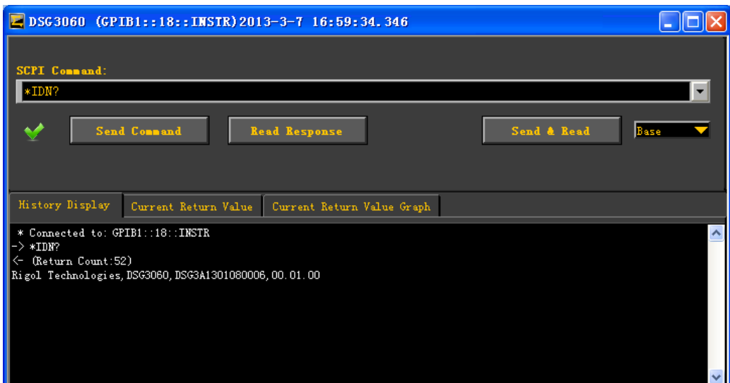
Figure 3-8 Write and read commands via GPIB
