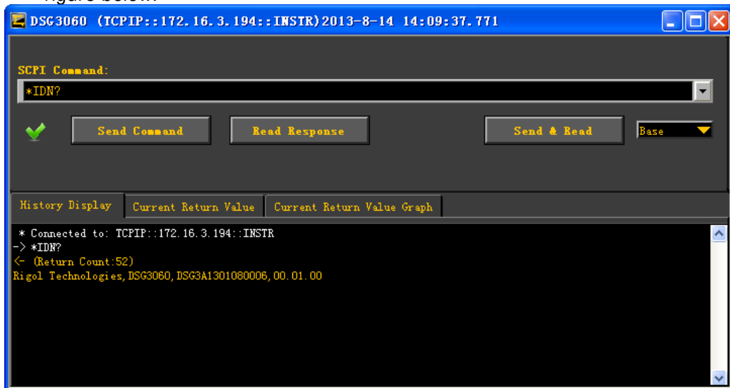
Figure 3-5 Write and read commands via LAN
