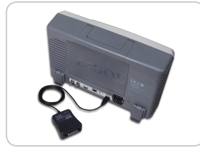
Optional USB-GPIB adapter for remote control
