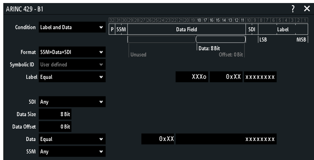
Figure 13-49: Settings for search on ARINC 429 bus
