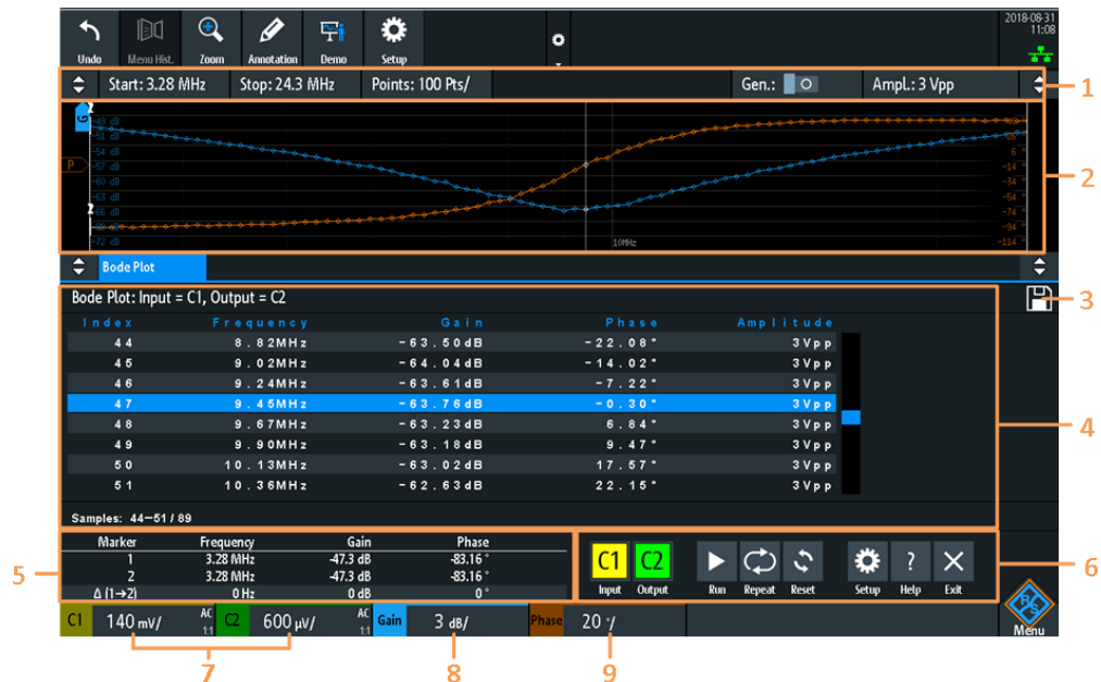
Figure 9-8: Bode plot display
