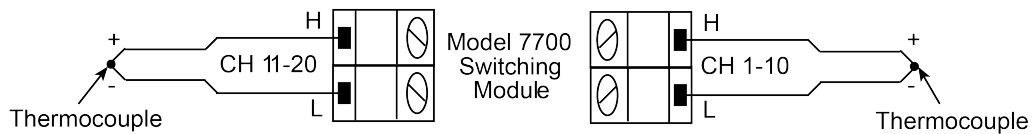
Figure 17: Channel average calculation, internal reference junction using a Model 7700
